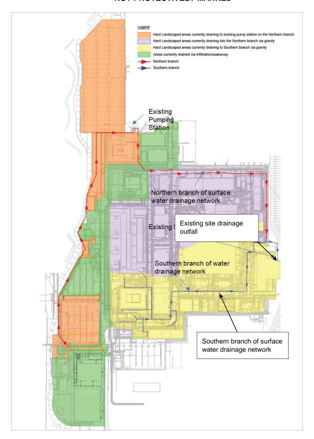
Figure 3-1: Existing Surface Water Drainage Network
