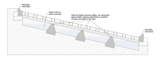
Figure 8-3: Permeable Paving Concrete Baffles [Marshalls- Permeable Paving Design Guide]
