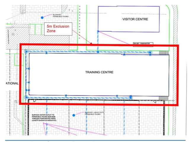
Figure 7-3:Infiltration Systems 5m Exclusion Zone
