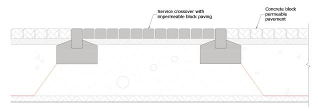
Figure 8-4: Impermeable and Permeable Paving
