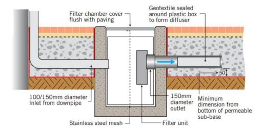
Figure 7-2: Discharge into Permeable Paving Sub Base
