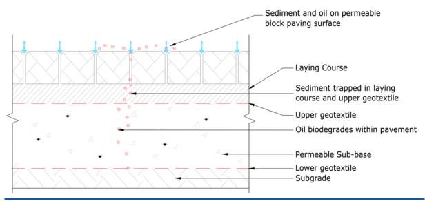
Figure 8-5: Permeable Sub-base Replacement System located beneath permeable paving structure [Interpave – Permeable Pavements]
